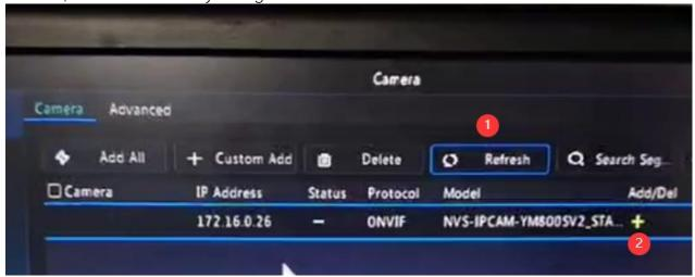
Third, after all IP address changed correctly into **192.168.2.xx**, let's select checkbox of camera And then select "Delete", this step is to delete all the cameras that been added, and then click "**Refresh**", and "**Add all**" again.
