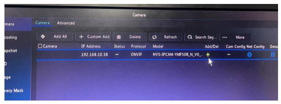
After adding camera into the system, the IP address will be changed into 192.168.2.xx and the status will change into blue icon, like picture below.
